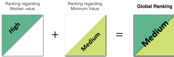
Figure 1: Illustration of the global ranking of Daylight Provision by aggregating the partial rankings reached for Median and Minimum values, CEN (2018).
